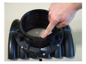
5. Lubricate the inner part of the rubber-part and the inner pipe-end.
