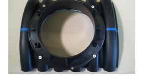
3. Put in the rubber-part. Crease it at the marked arrow and lift it until the rubber-part is closed fit at the inner-side of the pipe and the rubber edge is above the edge of the plastic part.
